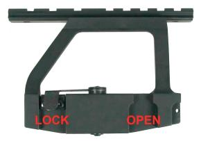
Once you have a snug fit with the adjustable mount you can slide the rail on from the back of the rifle. Have the throw lever 'open' and slide to the desired spot and then move the lever to the 'lock' side to secure.
