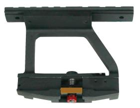
The mounting system is adjustable. The orange bracket will press against the rail on the side of the rifle. The red nut is able to be tightened to ensure a tight fit. To adjust the fitting you will have to press the orange section up and manually turn the red nut to fine tune the mount.
